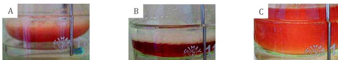
**Figure 5-8: Photos of the IO@RB synthesis A) the brown turbid solution during the water/oil emulsion at the 2<sup>nd</sup> step B) the black transparent solution after chloroform evaporation at the 3<sup>rd</sup> step C) the solution after the addition of all reactants at the 5<sup>th</sup> step**
