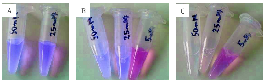
Figure 4-33: Photographs of second trial of silica dissolution by NaOH at various concentrations: 50, 20 and 5 mM; photographs were taken A) directly after NaOH addition, B) after 10 min, C) after 1 h
