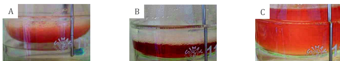
Figure 5-8: Photos of the IO@RB synthesis A) the brown turbid solution during the water/oil emulsion at the 2 nd step B) the black transparent solution after chloroform evaporation at the 3 rd step C) the solution after the addition of all reactants at the 5 th step
