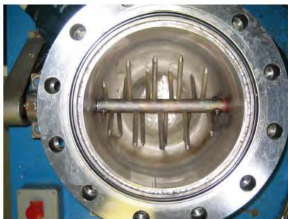
Figure 1-14. The inner chamber of the laboratory peg mixer (Zhang, Qin et al. 2009)
