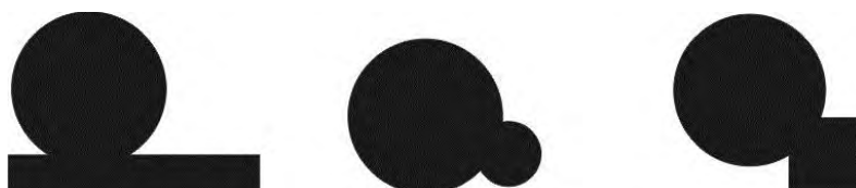
Figure 2-12. Illustration for particles in contact with lightning trace.
