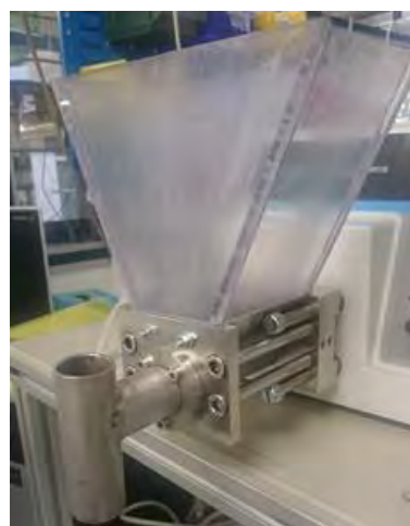
Appendix 6. Archimedean screw pump for substrate feeding: pump hopper, pump head, Archimedean screw and others disassembly parts
