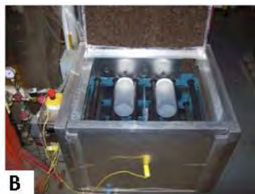
B Roller bottle reactor (RBR) (Roche, Dibble et al. 2009a, Roche, Dibble et al. 2009b)
