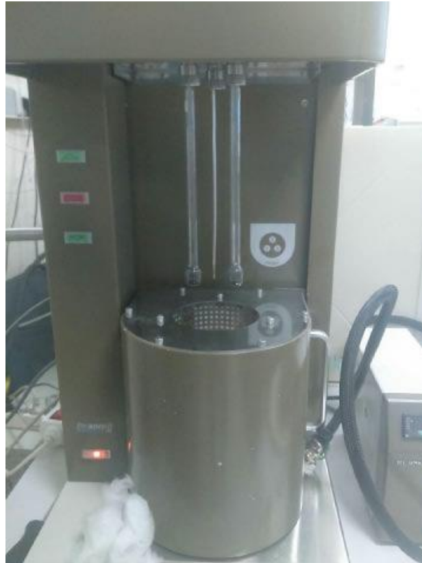
Figure 30: Nitrogen adsorption-desorption measuring device Belsorp-mini II (BEL Japan, Inc)
