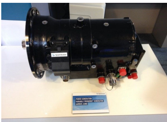
Figure 1-8 Illustration d'un Variable Frequency Generator [12]
