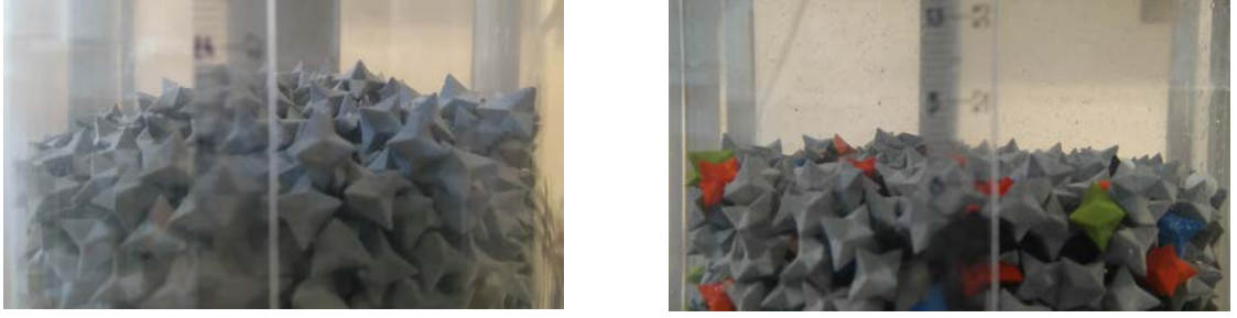
Figure 3.6: Upper surface of the equiaxed dendritic packed bed: Left) convex surface with dry protocol. Right) flat surface with glycerol protocol.
