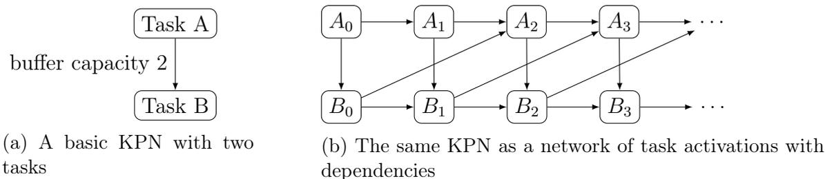
Figure 6.1: An example of decomposing KPNs into task activations
