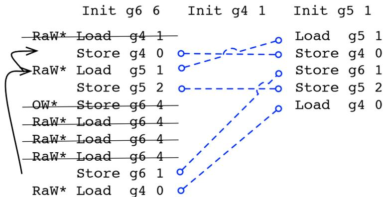
All the events in the optimized trace can be matched with events in the reference trace by performing valid eliminations and reorderings of events. Eliminated events are ~~struck-off~~ while the reorderings are represented by the arrows.
