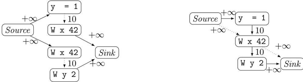
In the flow-graph on the left, the min-cut procedure finds a cut of finite weight (shown by the dotted lines). The edges in this cut are exactly where the fences are in the original program, so the optimisation correctly recognise that the program cannot be optimised.
