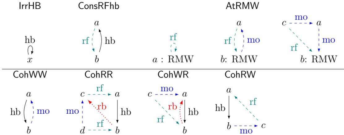
Figure 3.4: Executions violating the coherence axioms: all contain a cycle in  $\{(a, b) \in hb \mid loc(a) = loc(b)\} \cup com$ .
