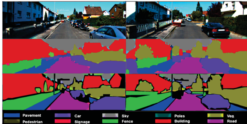
Figure 2.10 – Semantic image segmentation : The top row shows the input street-level images and the middle row shows the output of the CRF labeller. The bottom represents the ground truth. Source: (Sengupta et al., 2013).
