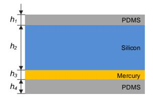
Figure 4.3 Layout of PDMS/silicon/mercury/PDMS film without pattern. The height of the mercury layer is  $h_3 = 50 \ \mu m$ ; the height of the bottom PDMS layer is  $h_4 = 1 \ mm$ .
