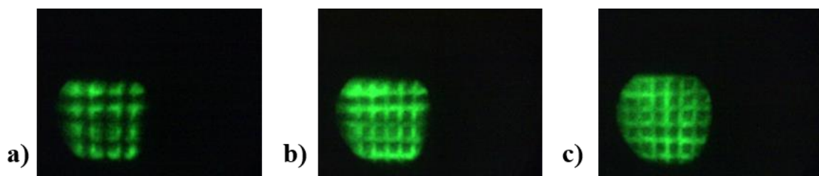
Figure 5. 42: Images of the grid with different raster sizes made with the 16 x 11.33 \mu\text{m} multi-hole aperture; a) 15 \mu\text{m} (10 fps); b) 25 \mu\text{m} (3 fps); c) 50 \mu\text{m} (3 fps).
