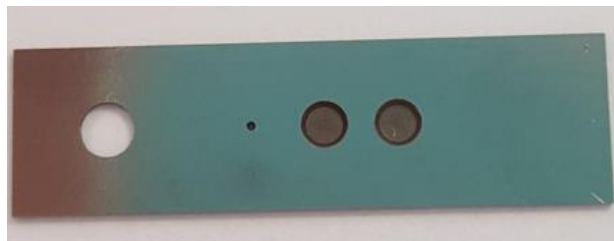
Figure 5. 29: Photo of the thin foil with the aperture of 200 \mu\text{m} , and the two multi-hole apertures described in Figure 5. 28.
