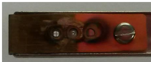
Figure 5. 19 : Aperture holder with three slots for 3 apertures, the hole with the cross corresponds to the 1mm aperture with the TEM grid superimposed.
