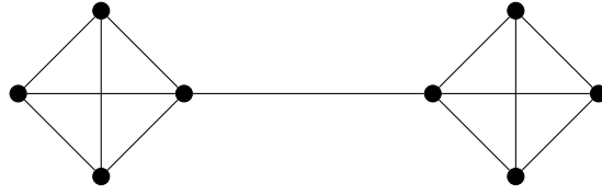
Figure 4.9: An example of a graph in which all 2-community structures are balanced
