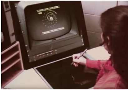
Figure 8. -Ron Baecker's Genesys. Built in 1969, it is the first digital tool explicitly designed to support animators' practices.
