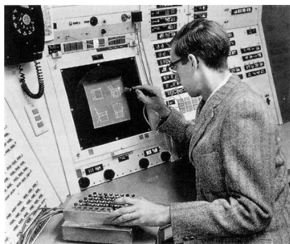
Figure 7. -Sutherland’s Sketchpad system. Built in 1963, it is considered to be the first visual interface and, coincidentally, the first digital design tool
