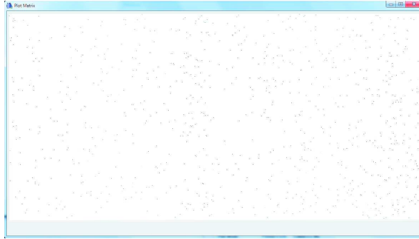
Figure 5.12 – Accumulation of 10^4 events at a threshold of 5 times the noise acquired in the dark for one sensor.
