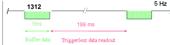
Figure 2.2 – Schematic view of the bunch structure at the ILC. One bunch train is made of 1312 bunches and lasts 1 ms long. Each bunch crossing is spaced out by 760 ns. Two bunch trains are 199 ms apart from each other [59].
