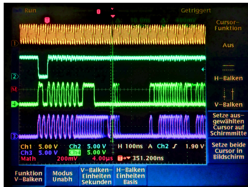
Figure 5.6 – MIMOSA-26 output from oscilloscope. The top yellow line corresponds to the clock, the blue line below to the marker (which lasts 4 clock cycles), and the green and purple lines are the data output containing the hit information
