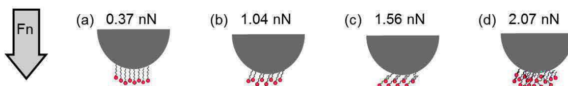
Figure 4.10. Schematics representing changes of the molecular structure under the increase of normal force ( F_n ). (a) For F_n=0.37 nN the layer keeps its stability and the molecules retain their perpendicular orientation towards the surface. (b, c) At F_n=1.04 nN and F_n=1.56 nN the passage of the AFM tip causes a molecular tilting. (d) For F_n=2.07 nN the pressure exerted by the tip is high enough to induce an order – disorder transition. Similar effects are expected on all CTAB film thicknesses. For 1 BL, however, the transition seems to occur at higher normal force values.
