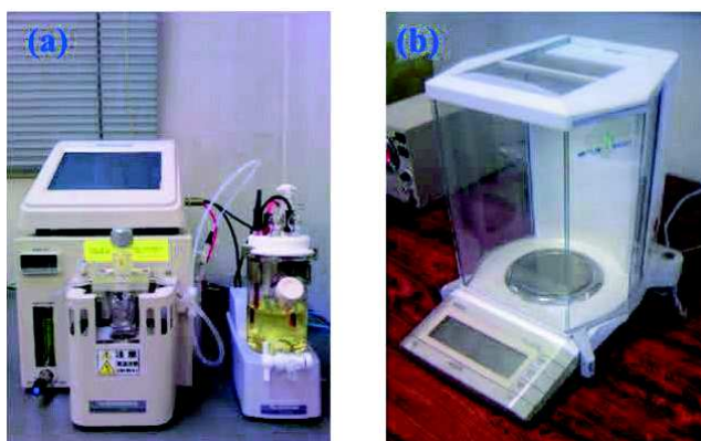
Fig. 2.3.1. Karl Fischer Coulometric Titrator, EV-200 (a), and electronic balance, AG245 (b),.
