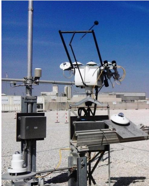
**Figure 37.** Weather station at the STF test site used to record wind speed and relative humidity. A separate, nearby particulate monitor was used for dust concentration measurements
