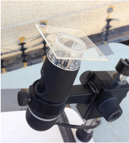
Figure 29. The outdoor soiling microscope (OSM) comprised a portable low-power microscope with a glass coupon glued to its front
