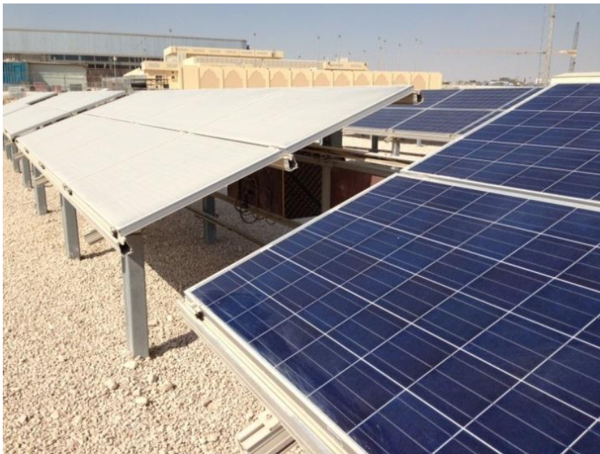
Figure 1. Cleaned and un-cleaned PV modules at the Solar Test Facility in Doha, Qatar. The study aimed to improve understanding of how soiling and condensation form on ambient surfaces in desert environments, via a novel outdoor microscopy
