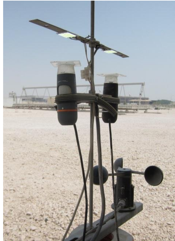
Figure 30. In many experiments a pair of OSMs was used to compare soiling on “treatment” and “reference” coupons in identical environmental conditions
