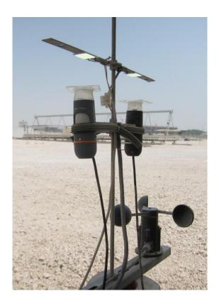
**Figure 30.** In many experiments a pair of OSMs was used to compare soiling on "treatment" and "reference" coupons in identical environmental conditions
