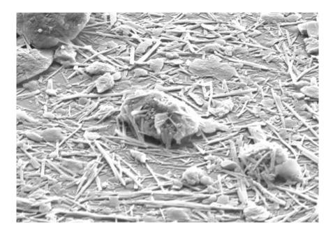
**Figure 24.** Needles of palygorskite following condensation on a soiled glass coupon at the STF, which visibly "cement" dust particles to the surface. The dust grain at the center of the image is  $\sim$ 1.5 µm long. Photo courtesy of Klemens Ilse, Fraunhofer CSP, Germany.
