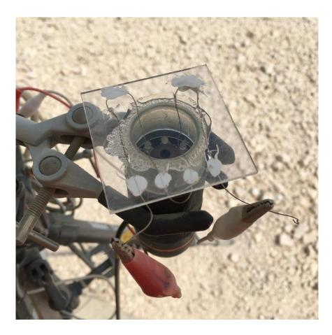
**Figure 69.** A heated OSM coupon was constructed using resistive nichrome wire. Its measurements were compared to those of an adjacent unheated coupon, to quantify the effect of condensation on dust flux rates in ambient conditions
