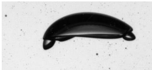
Figure II.20: Coalescence of a large and small bubbles in Breox (24%)
