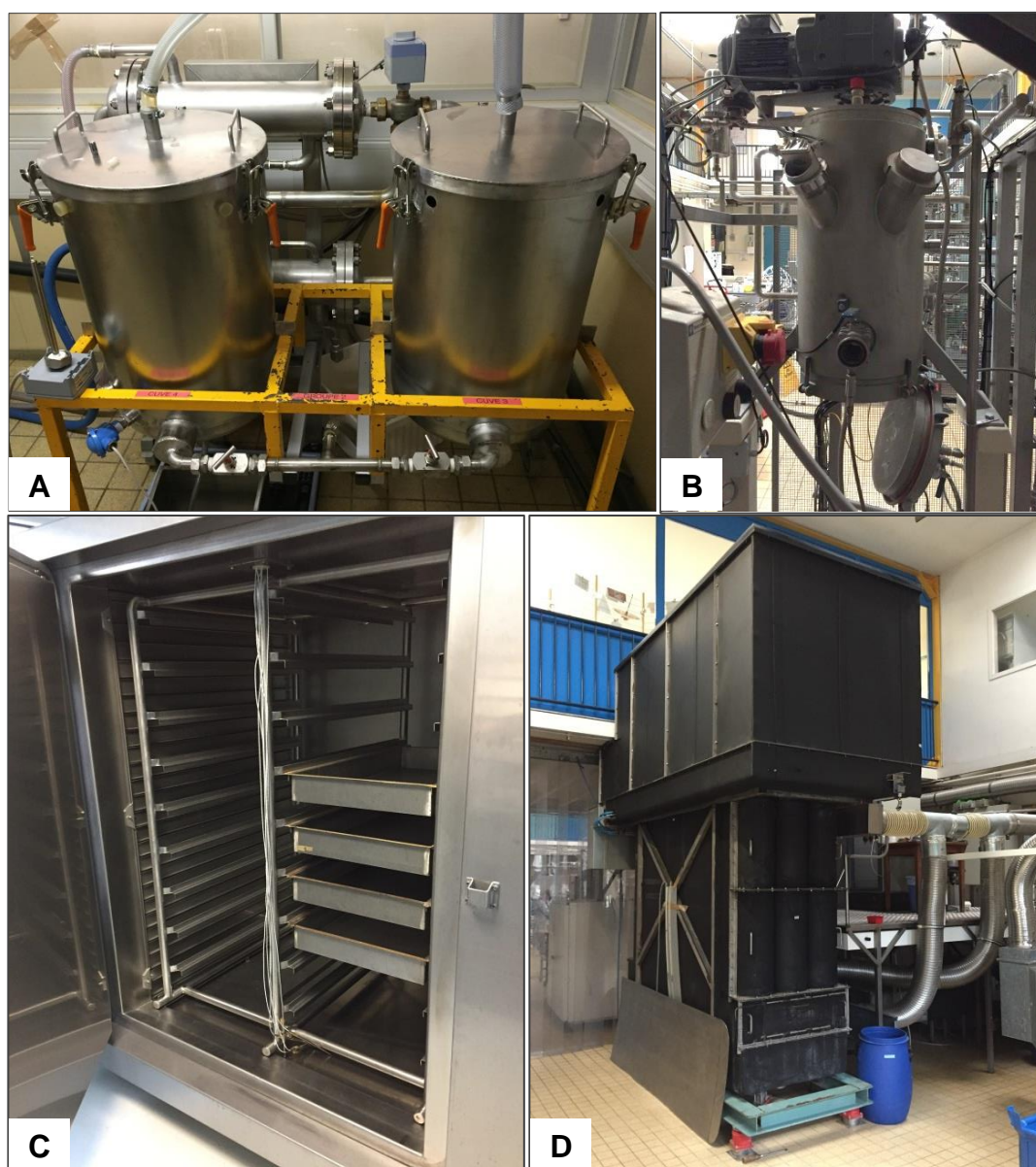
Fig. 4 Some pre-pilot and pilot-scale bioreactors at PPB, Dijon. (A) Packed-bed bioreactor, (B) sterile reactor of 50 L developed at PPB, (C) Koji-type reactor, 18 trays (D) Pilot plan reactor of 1.6 m 3 developed at PPB.
