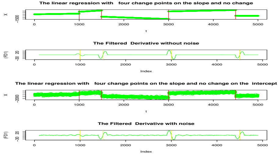
FIGURE 2.16 – First drawing : The observed signal, the third drawing : The Filtered derivative function for the slope without noise, the fourth drawing : The Filtered Derivative with noise.
