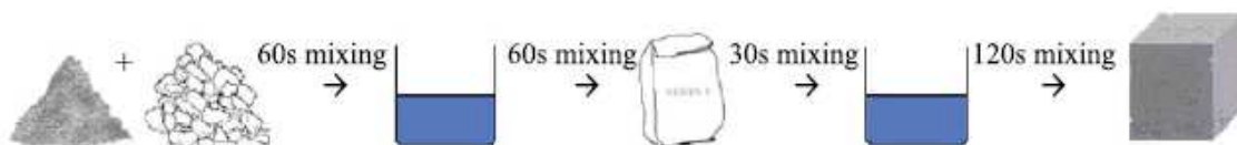
Figure 1- 8: TSMA two steps mixing approach (Tam et al., 2005) ; 4 mn 30 de malaxage au total
