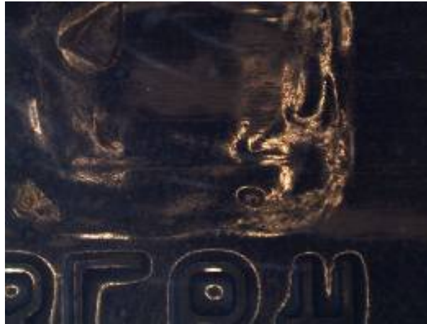
Figure 6.2: Deformation due to heating of the forgery's backside.
