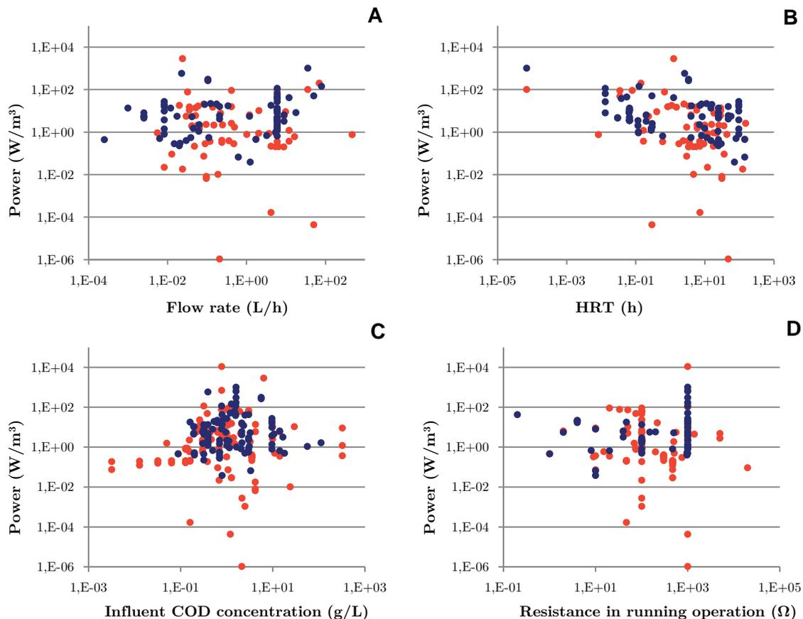
**Figure 14.** Anodic volume power density vs different MFCs operational parameters: Flow rate (A), Hydraulic retention time (B), Influent COD concentration (C), external resistance (D) (red dots: data from operating MFC; blue dots: data from polarization curve).
