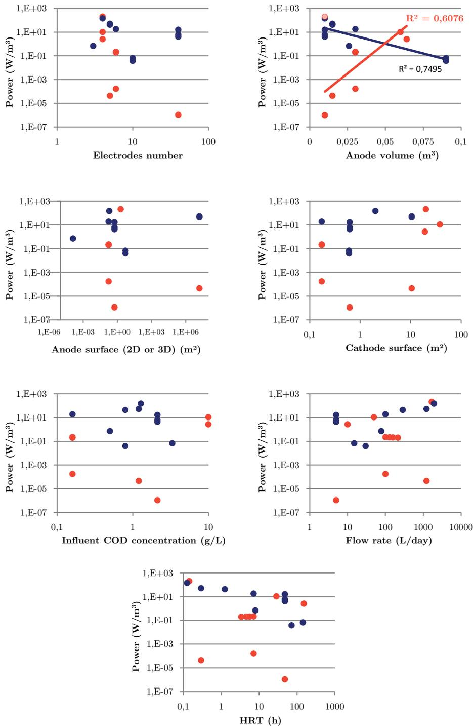
Figure 9. Anode volumetric power density vs different parameters for MFCs larger than 10L (red dots: power while MFC is operating; blue dots: maximal power in polarization curve). The second panel (power vs anode volume) shows the linear regression lines for the data while MFC is operating (red dots) without the eccentric point (light red dot) and from polarization curves (blue dots).
