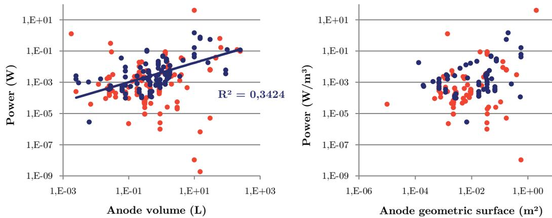
**Figure 10. Power vs anode compartment volume and anode geometric surface (red dots: power while MFC is operating; blue dots: maximal power in polarization curve). The first panel (power vs anode volume) shows the linear regression line for the data from polarization curves (blue dots).**
