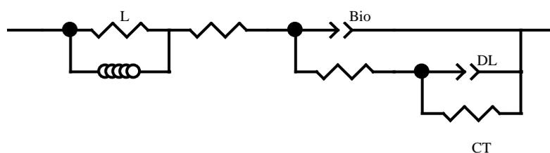
**Figure 19. Electrical equivalent circuit used to fit anode impedance spectra. L: inductance;  $R_L$ : resistance from inductive behavior;  $R_{ohm}$ : electrolyte resistance;  $R_{CT}$ : charge transfer resistance;  $R_{Bio}$ : biofilm resistance;  $CPE_{DL}$  &  $CPE_{Bio}$ : constant phase elements respectively from double layer and biofilm.**
