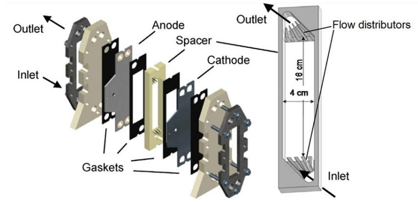
Figure 15. Filter-press reactor (modified from Rivero *et al.*<sup>128</sup>).
