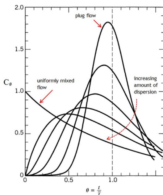
Figure 18. Hypothetical tracer response curves varying from plug flow to uniformly mixed flow reactors as adapted from Levenspiel<sup>130</sup>;  $\theta$  is a dimensionless time unit  $\theta = t/\bar{t}$  and  $C_\theta$  is the tracer concentration in function of  $\theta$ .
