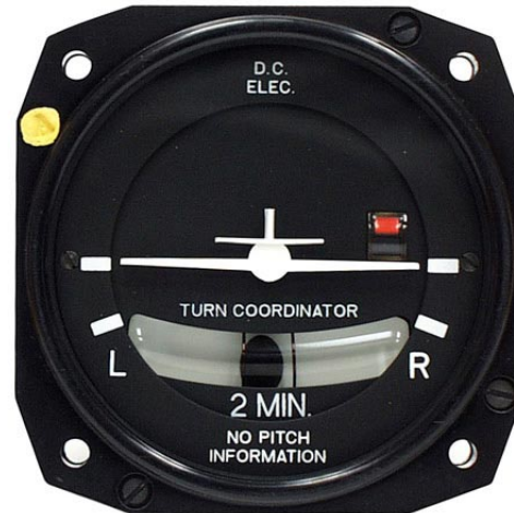
FIGURE 8.12: Slip/Skid Indicator for turn coordination. The ball to the right indicates slip and to the left indicates skid. Only gravity forces affect the ball position (CFI, 2017).
