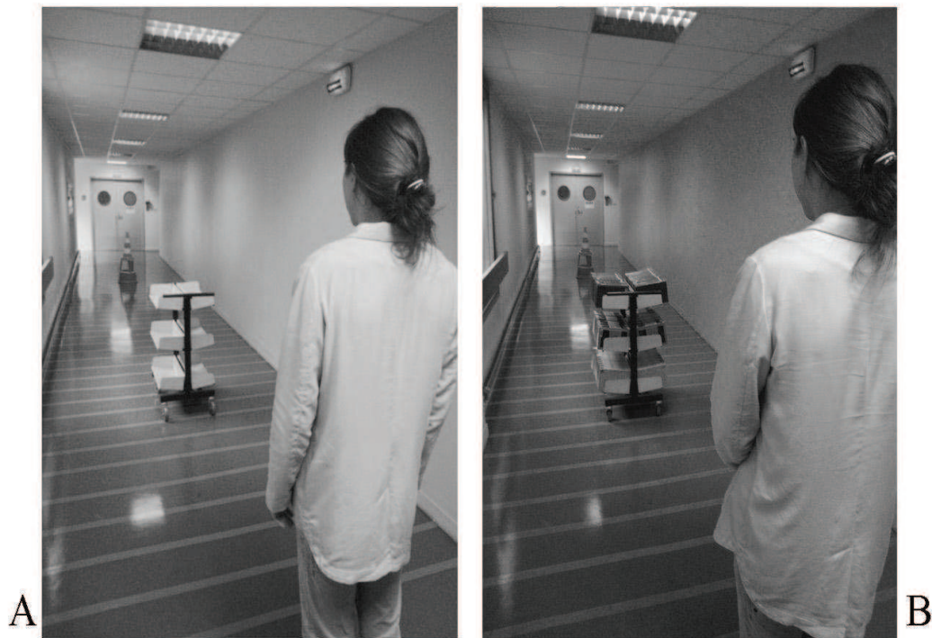
Figure 2.1 – Experimental apparatus from the participants’ perspective for the light group (A) and the heavy group (B). These pictures represent the near condition, with the trolley located 3 m from the participant and the cone (target) located 8 m away from the trolley
