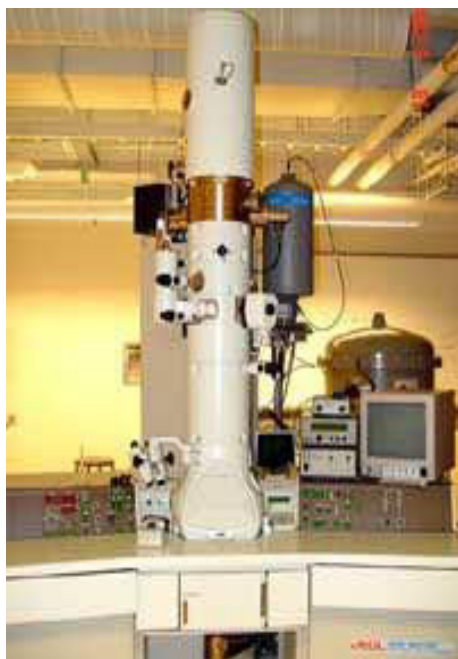
Figure 4 Scheme of electron transmission microscope
