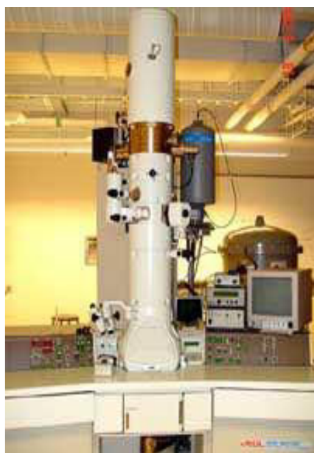
Figure 4 Scheme of electron transmission microscope
