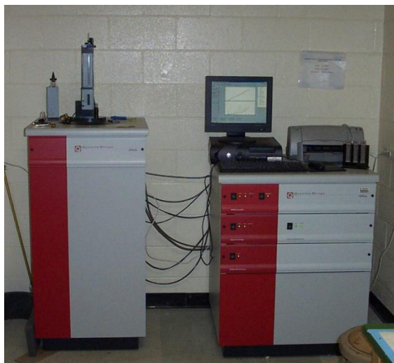
Figure 6 SQUID instrument and schematic representation
