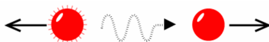
Figure II.1 Recoil of free nuclei in emission or absorption of a gamma ray
