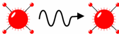
Figure II.3 Recoil-free emission or absorption of a gamma-ray when the nuclei are in a solid matrix such as a crystal lattice
