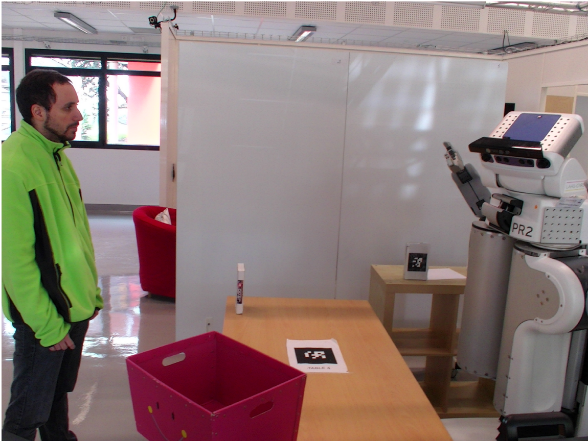
FIGURE 8.1: The robot coworker scenario example, with a PR2 robot and a user.
