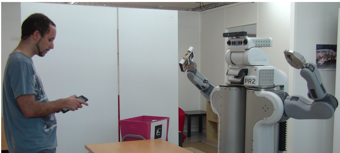
FIGURE 6.3: The human is giving a goal to the robot by using a tablet application.
