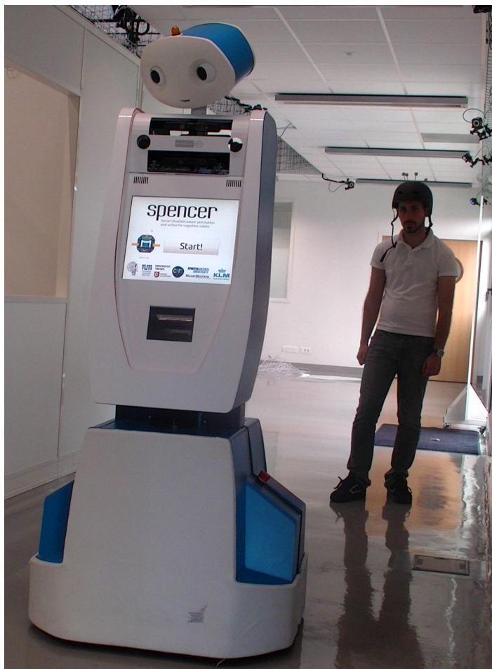
FIGURE 13.1: This figure shows the SPENCER robot guiding a user in a laboratory.
