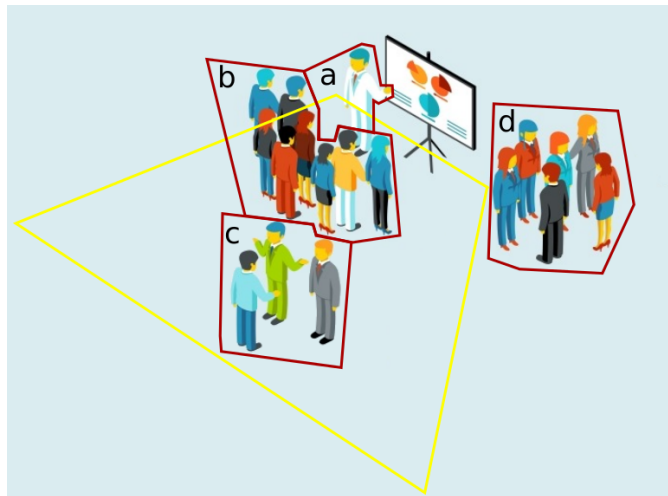
FIGURE 12.2: The Information Screen area used for environment-based intention recognition. The yellow polygon represents an area linked to the screen in the figure. Red polygons represent groups of persons in the area. The person in group a is in the screen area, but the robot will infer that he is not looking at the screen, since he is oriented in another direction. The persons in group b are in the screen area and oriented toward the screen, so the robot infers that they are looking at it. The persons in group c are not looking at the screen since they are either oriented in another direction or outside its area.
