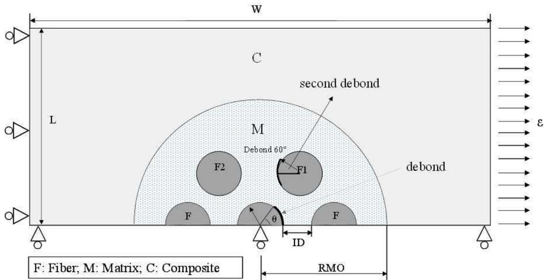
**Fig.30** Schematics of the model used for debond growth analysis around the central fiber showing explicitly the central fiber and the 6 closest fibers. One of them may have a Semi-angle of  $60^\circ$  debond on one side. The fiber/matrix unit is embedded in a homogenized composite.
