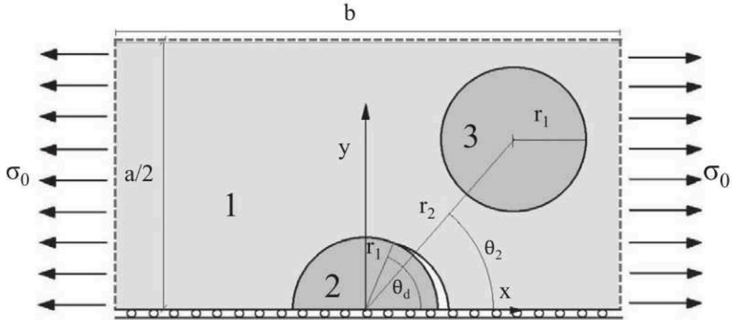
**Fig.16** Illustration of two fibers numerical model. Figure adopted from [112]
