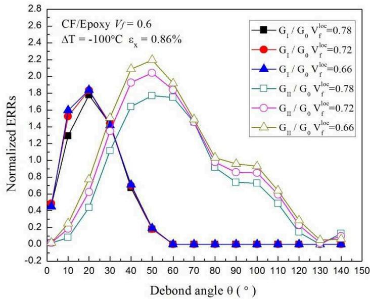
Fig. 9. Normalized ERR with respect to debond angle for CF/EP UD plies, equivalent to 90-layers of CF/EP cross-ply laminate under thermo-mechanical loading.  $V_f = 0.6$ ,  $\Delta T = -100^\circ\text{C}$ ,  $\varepsilon_x = 0.86\%$
