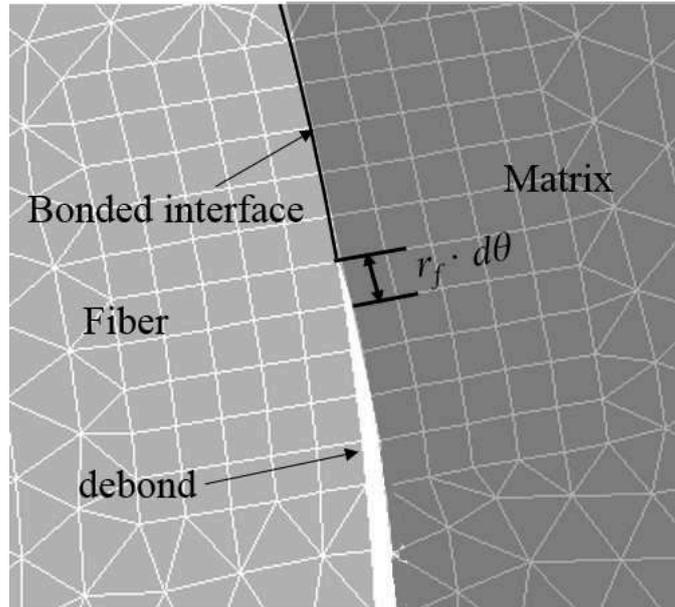
Fig.2 Details of mesh near debond tip
