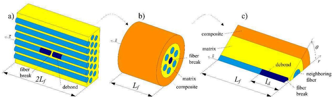
**Fig. 21** a) UD composite with a broken and partially debonded fiber; b) Hexagonal distribution model; c) unit cell  $\theta=30^\circ$
