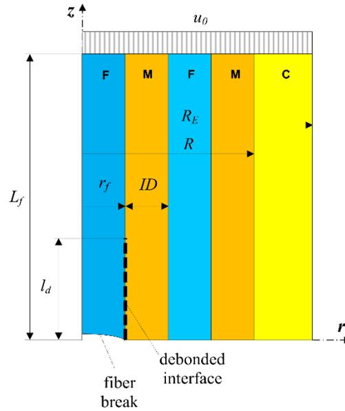
**Fig.18** Schematic representation of a 5-phase concentric cylinder assembly FEM model for short debond energy release rate calculations: F –fiber, M – matrix, C – effective composite.
