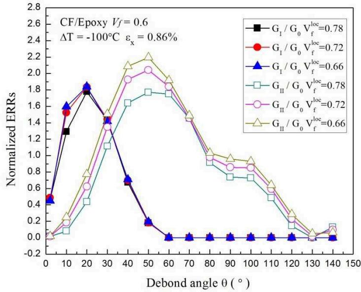
**Fig. 29** Normalized ERR with respect to debond angle for CF/EP UD plies, equivalent to 90-layers of CF/EP cross-ply laminate under thermo-mechanical loading.  $V_f = 0.6$ ,  $\Delta T = -100^\circ\text{C}$ ,  $\epsilon_x = 0.86\%$
