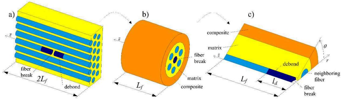
Fig. 1. a) UD composite with a broken and partially debonded fiber; b) Hexagonal distribution model; c) unit cell  $\theta=30^\circ$
