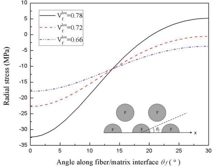
Fig. 8. Radial stress distribution along bonded fiber/matrix interface due to thermal cool-down,  $\Delta T = -100^\circ\text{C}$ .
