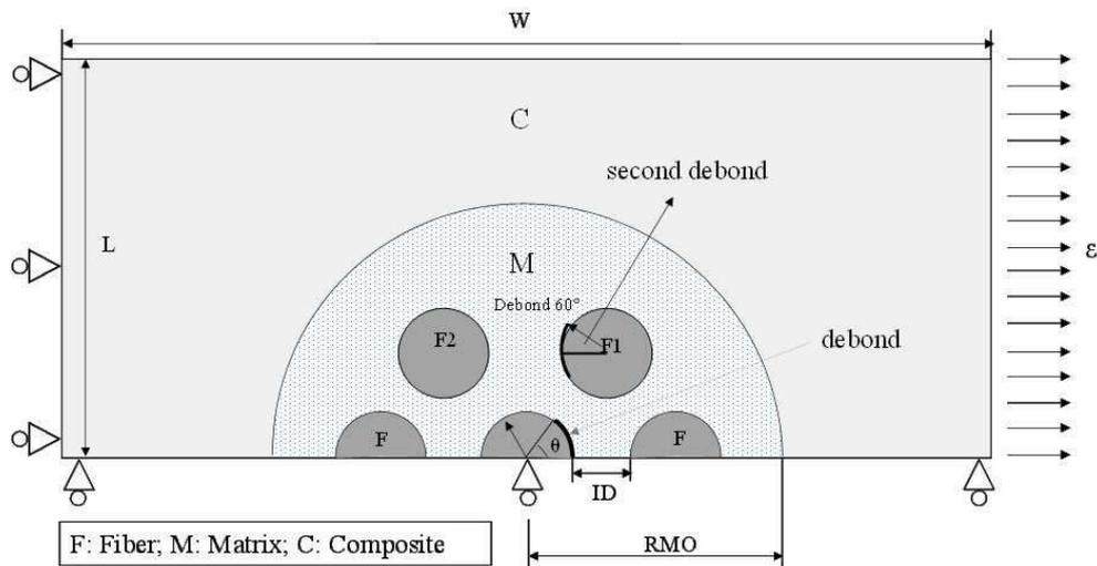
**Figure 1.** Schematics of the model used for debond growth analysis around the central fiber showing explicitly the central fiber and the 6 closest fibers. One of them may have a Semi-angle of  $60^\circ$  debond on one side. The fiber/matrix unit is embedded in a homogenized composite.
