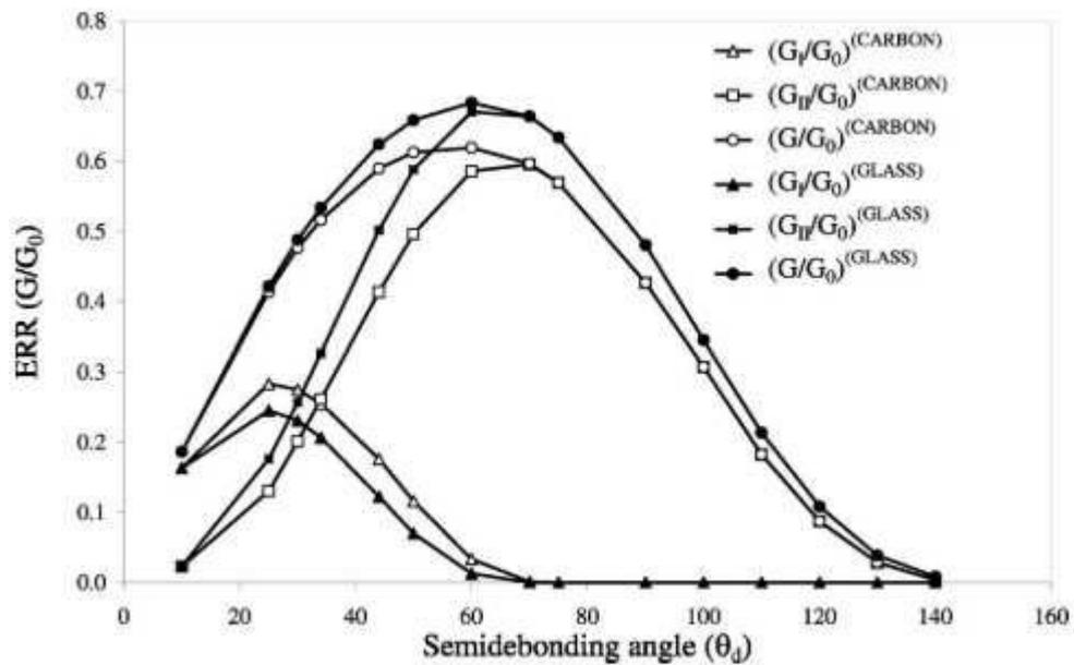
**Fig.15** Illustration of the trend for ERR of the debond in a single fiber composite. Figure adopted from [101]
