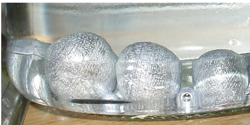
Figure 1.1: Potassium balls stored in oil to prevent reaction with water vapour in air.
