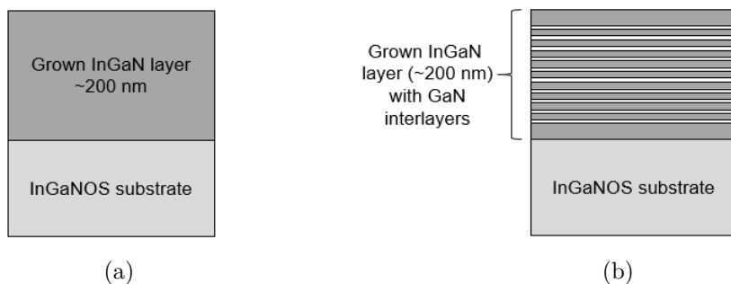
FIGURE 4.18 – Structures of InGaN layers on InGaNOS. The reference is on the left (a). For the second structure, 10 GaN interlayers of 2 nm were regularly placed in the InGaN layer (b).
