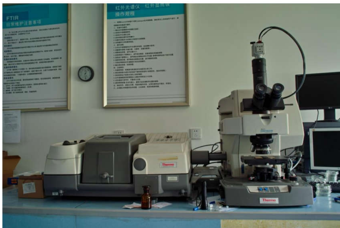
Fig. 3-2 Picture of the Nicolet 5700 FTIR spectrometer coupled with a microscope, located at USTC
