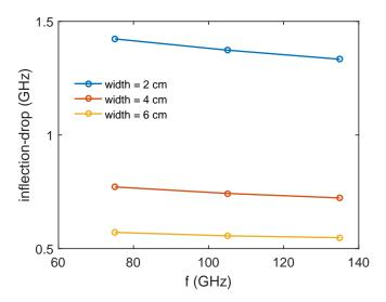
Fig. 4.12 The drop in amplitude observed for varying peak widths and probing frequencies at the sweeping rate of 20 GHz/ $\mu$ s.
