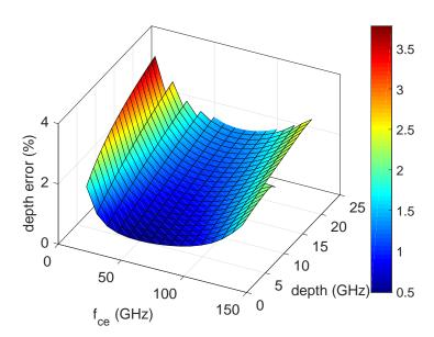
Fig. 4.41 Error in estimated perturbation depth for a 1 GHz error in  $f_{ce}$ . The remaining parameters are kept constant, with width = 4.5cm,  $f_{end} = 160GHz$  and  $\nabla f_R = 82GHz/m$ .
