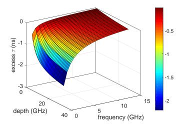
Fig. 4.31 Example solution of database of time-of-flight excess signals for sine shape valleys in the fixed conditions of width = 2cm,  $f_{end} = 126.2GHz$ ,  $f_{ce} = 12.5GHz$ ,  $\nabla f_R = 118GHz/m$ .
