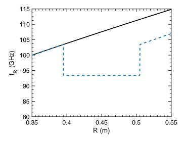
Fig. 4.15 Square perturbation to investigate the uniformity of the time-of-flight contribution across the perturbation.
