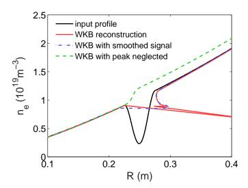
Fig. 4.1 Input and reconstructed density profiles containing a blind region. The profile was reconstructed with the standard Bottollier-Curtet algorithm with W=2/3 using three different treatments in the phase signal.
