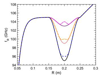
Fig. 4.22 Profiles with  $\sin^2$  perturbations of varying depths, with and without an additional  $\delta f_R$  of constant area. The plateau before the perturbation is introduced to decrease the frequency bandwidth tunnelled into the perturbation Doing so reduces the interferences, and therefore, reduces the fluctuations on the time-of-flight signal.
