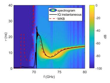
Fig. 5.15 Time-of-flight signals corresponding to frequency profiles of Fig. 5.13, top case, swept at 20 GHz/ $\mu$ s. The perturbation is inserted at 0.06 m and is directly probed in the frequency range between approximately 68 and 69.8 GHz.
