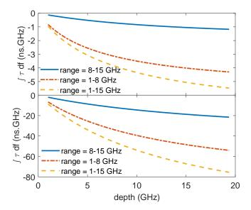
Fig. 4.34 Different ranges in the time-of-flight integration for two solution conditions. Top case with width = 2cm,  $f_{end} = 47.5GHz$ ,  $f_{ce} = 24.9GHz$  and  $\nabla f_R = 106GHz/m$ . Bottom case with width = 9.7cm,  $f_{end} = 227.5GHz$ ,  $f_{ce} = 199GHz$  and  $\nabla f_R = 106GHz/m$ .
