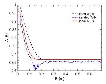
Fig. 3.10 Ideal and estimated integration factors W(R). The fitted case assumed one at the first probing frequency and goes linearly to 2/3 at the pedestal position assumed at 0.22 m. The iteration process already converges after the first iteration, not changing significantly with further iterations. The input frequency profiles are the same as in Fig. 3.3 but with the pedestal moved to 0.175 m.
