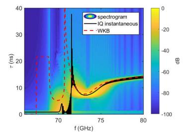
Fig. 5.16 Time-of-flight signals corresponding to frequency profiles of Fig. 5.13, middle case, swept at 20 GHz/ $\mu$ s. The perturbation is inserted at 0.10 m and is directly probed in the frequency range between approximately 68.8 and 70.8 GHz.
