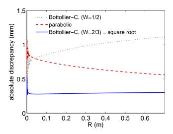
Fig. 3.5 Profiles of absolute radial discrepancy when reconstructing the density profile with the conditions of linear  $f_R$  profile, 500 probing frequencies and a precision of 0.1 mm in the initialization.
