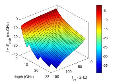
Fig. 4.40 Surface of integrated time-of-flight showing the impact in depth related to  $f_{ce}$ . The remaining parameters are kept constant, with width = 4.5cm,  $f_{end} = 160GHz$  and  $\nabla f_R = 82GHz/m$ .
