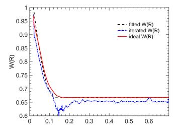
Fig. 3.9 Ideal and estimated integration factors W(R). The fitted case assumed one at the first probing frequency and goes linearly to 2/3 at the pedestal position assumed at 0.13 m. The iteration process already converges after the first iteration, not changing significantly with further iterations. The input frequency profiles are the same as in Fig. 3.3 but with the pedestal moved to 0.175 m
