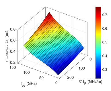
Fig. 4.37 Accuracy as given in Eq. 4.6, averaged over all depths  $d_v$ , for the fixed parameters of  $f_{end} = 197GHz$ , width = 2cm, showing dependency on  $f_{ce}$  versus  $\nabla f_R$ .
