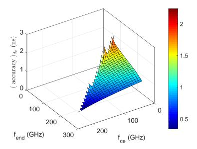
Fig. 4.39 Accuracy as given in Eq. 4.6, averaged over all depths  $d_v$ , for the fixed parameters of  $\nabla f_R = 34GHz/m$  and width = 16cm, showing the dependencies on  $f_{end}$  versus  $f_{ce}$ .
