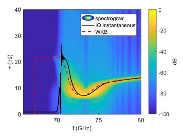
Fig. 5.12 Time-of-flight signals corresponding to the unperturbed profiles of Fig. 5.11, with a sweeping rate of 20 GHz/ $\mu$ s.
