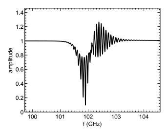
Fig. 4.9 IQ amplitude crossing a narrow barrier of 1 cm and jumping over a 40 cm wide perturbation. The probing frequency is swept at 20  $GHz/\mu s$ .
