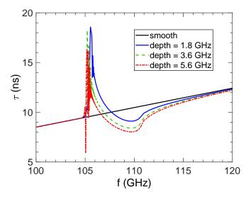
Fig. 4.6 Time-of-flight signals from the profiles introduced in Fig. 4.5, calculated with the IQ method as presented in section 1.3.1. The sweeping rate used was 20 GHz/ $\mu$ s.
