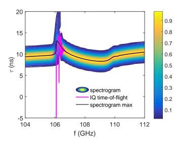
Fig. 4.14 IQ spectrogram and instantaneous frequency signals with a negative resonance case. The profiles used are the standard study case resulting in background density of  $3 \times 10^{19} m^{-3}$  and magnetic field of 3 teslas at the perturbation location. The perturbation introduced has a sine square shape with 14 cm width and depth in the density profile of  $0.66 \times 10^{19} m^{-3}$ .
