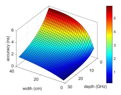
Fig. 4.36 Reconstruction accuracy computed according to Eq. 4.6. All other parameters are fixed at  $f_{end} = 167GHz$ ,  $f_{ce} = 91GHz$  and  $\nabla f_R = 82GHz/m$ . The accuracy is displayed versus the geometrical parameters depth and width.
