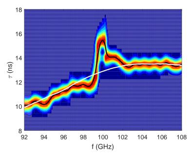
Fig. B.2 Time-of-flight signal around the perturbation of interest compared to the reference unperturbed case in white. Tore Supra discharge 32029, with the perturbation at t=3.0037 s and the reference unperturbed case at t=3.0033 s.
