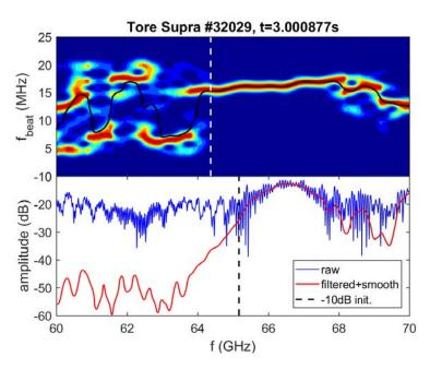
Fig. C.1 Top: spectrogram around the initialization frequency, bandpass filtered between 3 and 22 MHz. The white dashed line marks a drop of the broadband fluctuations. Bottom: the amplitude rise around the initialization frequency. The dashed black line marks the frequency that has amplitude of -10 dB compared to the top of the amplitude rise.
