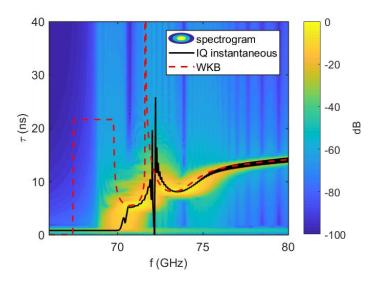
Fig. 5.17 Time-of-flight signals corresponding to frequency profiles of Fig. 5.13, bottom case, swept at 20 GHz/ $\mu$ s. The perturbation is inserted at 0.14 m and is directly probed in the frequency range between approximately 69.8 and 71.6 GHz.
