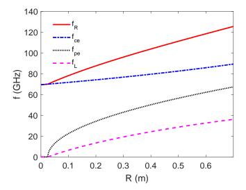
Fig. 1.11 The solutions obtained for the O-mode and X-mode cut-off profiles, based on the  $f_{pe}$  and  $f_{ce}$  profiles originating from the density and magnetic field profiles assumed in Fig. 1.10.
