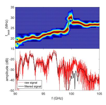
Fig. B.1 Beat frequency and amplitude signals around the perturbation to be investigated. Only a broad bandpass filter was applied to remove reflections that were far from the main branch. Tore Supra discharge 32029 at t = 3.0037 s.
