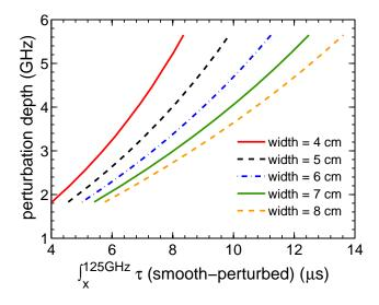
Fig. 4.26 Relations of hole depth to the integral of the time-of-flight difference between perturbed and unperturbed cases. The integral is computed from the probing frequency where the perturbed time-of-flight crosses the unperturbed case until 20 GHz above the frequency of the time-of-flight jump (in this case, 125 GHz).
