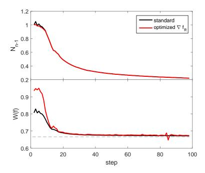
Fig. A.3 Comparison of two reconstruction parameters between two cases when using the originally computed  $\nabla f_R$  profile and when adjusting it by multiplying by 0.47. The parameters are related to the profile reconstructions in Fig. A.4 when using 100 frequency steps. At the top, the refractive index in the previous known position, and at the bottom, the optimized weight factors.
