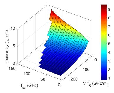
Fig. 4.38 Accuracy as given in Eq. 4.6, averaged over all depths  $d_v$ , for the fixed parameters of  $f_{end} = 197GHz$  and width = 32cm, showing the dependencies on  $f_{ce}$  versus  $\nabla f_R$ .
