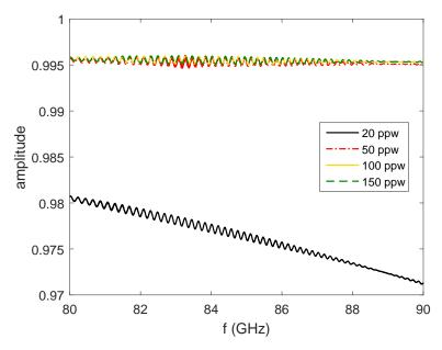
Fig. 2.1 Effect of numerical dispersion from the choice of the number of points per wavelength for the simulation of a linear density profile and  $50\,\mathrm{GHz/us}$  frequency sweeping rate.
