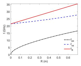
Fig. 3.16 Low density and magnetic field case with enforced linear profile in  $f_R$ , with  $\nabla f_R = 20\,GHz/m$ . This case represents the worst case scenario for the reconstruction algorithm if not optimizing the integration factors W.
