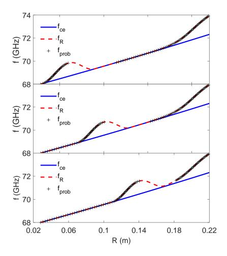
Fig. 5.13 Base frequency profiles of Fig. 5.11 with a perturbation inserted at three different radial positions. From top to bottom,  $R_{pert} = 0.06$ , 010 and 0.14 m. In the top case, above the perturbation, there is still a range of probing frequencies on the region with negligible plasma density. For the middle case, the jump frequency matches where it would be the unperturbed initialization frequency. At the bottom case, the frequency jump is already inside the main profile.
