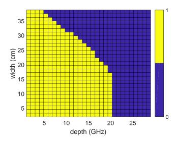
Fig. 4.32 Example of validity domain in database solutions for the fixed parameters of  $f_{end} = 70GHz$ ,  $f_{ce} = 37.3GHz$  and  $\nabla f_R = 118GHz/m$ . The valid solutions are numbered with the number one and displayed with the color yellow.
