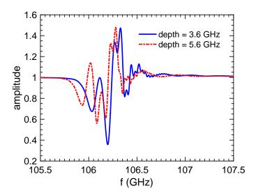
Fig. 4.8 IQ amplitude of sine squared valley perturbations as introduced in Fig. 4.5 but with width reduced to 4 cm. The probing frequency is swept at 20 GHz/ $\mu$ s.
