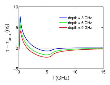
Fig. 4.30 The maximum of the IQ spectrogram time-of-flight signal when simulating the sweep on the profiles presented in Fig. 4.28.
