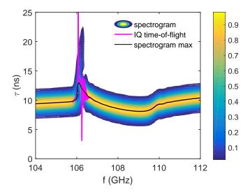
Fig. 4.13 IQ spectrogram and instantaneous frequency signals with a positive resonance case. The profiles used are the standard study case resulting in background density of  $3 \times 10^{19} m^{-3}$  and magnetic field of 3 teslas at the perturbation location. The perturbation introduced has a sine square shape with 5 cm width and depth in the density profile of  $0.66 \times 10^{19} m^{-3}$ .
