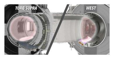
Fig. 1.7 Upgrade from Tore Supra to WEST. Left: The Tore Supra cross section, with carbon plasma facing components and a limited plasma configuration. Right: The WEST cross-section with tungsten plasma facing components and a diverted plasma configuration. From Ref. [17].
