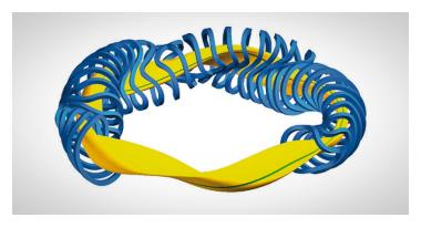
Fig. 1.5 Magnetic coils in blue and plasma shape in yellow for the stellarator Wendelstein 7-X. From Ref. [13].
