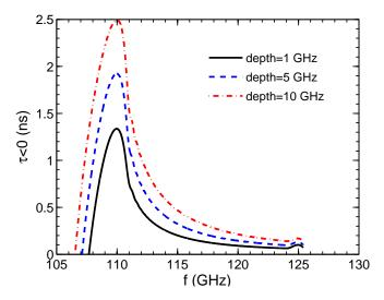
Fig. 4.25 Drop in time-of-flight from  $sine^2$  perturbations as introduced in Fig. 4.6, if subtracted by the smooth solution, starting when the signals with perturbation crosses the unperturbed solution.
