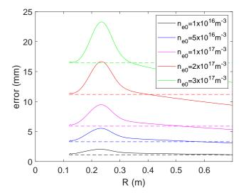
Fig. 5.6 Error profile when reconstructing the density profile using the optimized scheme of chapter 3 while skipping a shallow plasma 12 cm long with varying values of a constant density. The dashed lines represent the distance between  $f_R$  and  $f_{ce}$  for the initial probing frequency.
