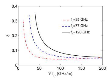
Fig. 3.15 The  $\delta$  parameter from index fitting shape as given by Eq. 3.19 versus the cut-off profile gradient.
