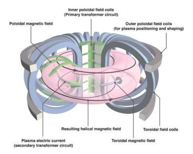
Fig. 1.6 The tokamak reactor design. The design is simplified due to the symmetrical coils and the poloidal field component is generated by the plasma current induced by the central transformer. The poloidal coils generate the toroidal magnetic field, while the toroidal coils are used to tune the plasma position. From Ref. [17]
