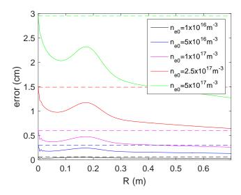
Fig. 5.3 Error profile when reconstructing the density profile using the optimized scheme of Chap. 3 with varying values in starting density,  $n_{e0}$ . The dashed lines represent the distance between  $f_R$  and  $f_{ce}$  for the probing frequency considered as the initialization point.
