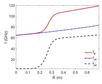
Fig. 5.1 Frequency profiles used as a base case for the benchmarks in Sec. 5.1. The density and magnetic field have magnitudes typical of Tore Supra discharges with a pedestal located around  $0.2~\mathrm{m}$ .
