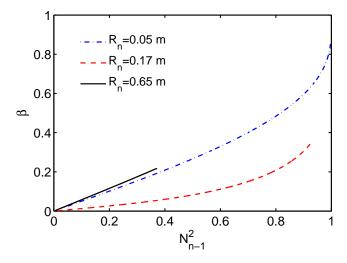
Fig. 3.13 The  $\beta$  parameter from the refractive index fitting shape given in Eq. 3.18, as a function of  $N_{n-1}^2$ , taken at three example radial positions for the example of typical Tore Supra profiles as given in Fig. 3.3.
