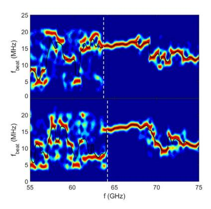
Fig. C.2 Comparison of the probing frequency where the broadband fluctuation decreases for two sweeps around  $t=3.02~\mathrm{s}$  at the Tore Supra shot 32029.
