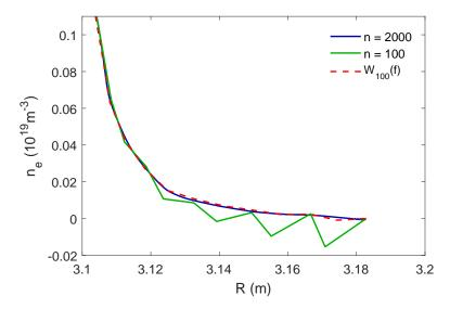
Fig. A.4 Comparison between edge density profiles when using 2000 or 100 frequency steps with the constant W=2/3 and also a case with 100 frequency steps with  $W(f_{prob})$  optimized for each probing frequency. In this case, the values of  $\nabla f_R$  used to compute  $W(f_{prob})$  have been multiplied by 0.47. Tore Supra discharge 32029 at t=3.0037 s.
