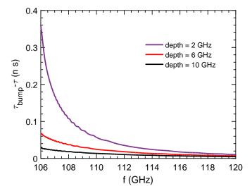
Fig. 4.24 Time-of-flight difference between valleys without and with a positive  $\delta f_R$  perturbation, as introduced in Fig. 4.22. The probing frequency range starts just after the jump in time-of-flight.
