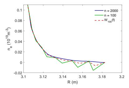
Fig. A.1 Comparison between edge density profiles when using 2000 or 100 frequency steps with the constant W=2/3 and also a case with 100 frequency steps with  $W(f_{prob})$  optimized for each probing frequency. Tore Supra discharge 32029 at t=3.0037 s.
