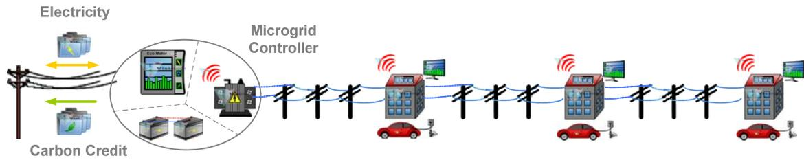
Figure 1.3 – Sample MG as a low voltage feeder [2].
