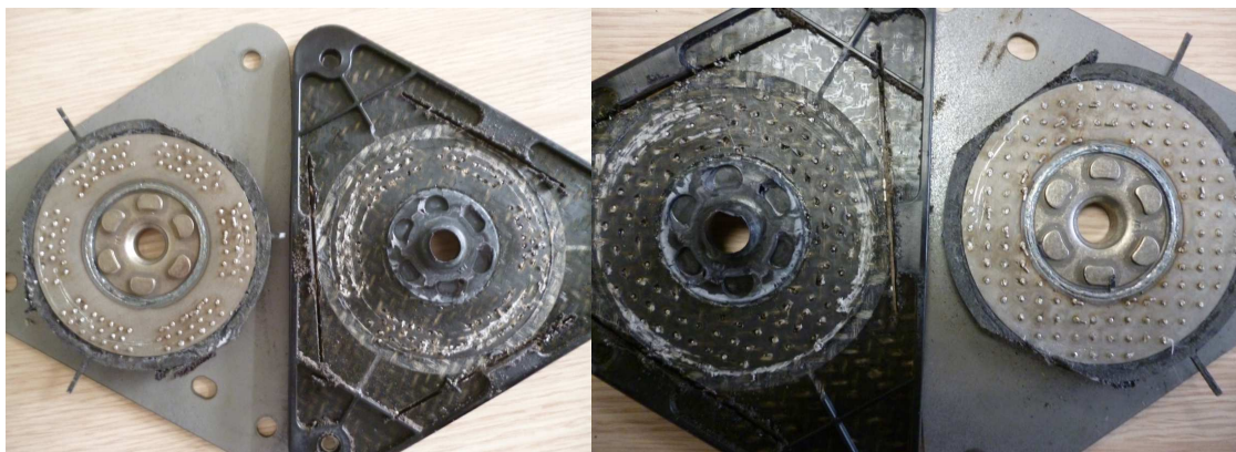
Figure IV.114. Aspect post rupture de l'interface
