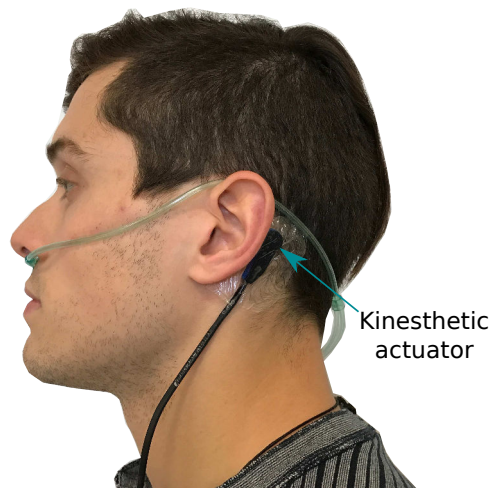
Figure 4.4: Placement site of the kinesthetic actuator. The selected region is on the mastoid bone behind the ear of the patient which is an area rich in mechanoreceptors, allowing a more effective activation of the startle reflex (see section 3.1.2).
