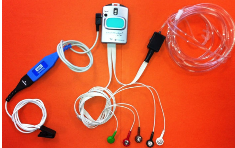
Figure 4.2: The prototype cardiorespiratory Holter device with associated sensors (ECG electrodes, SaO 2 ear sensor and nasal pressure cannula).
