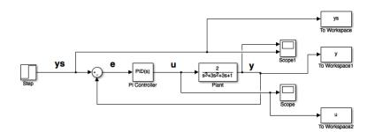
Figure 3.11: Block diagram of the previously mentioned example system in figure 3.4 implementing a proportional-integrative control. Being e the control error,  $y_s$  the target or expected value for the control variable, y the control variable and u the output of the controller.
