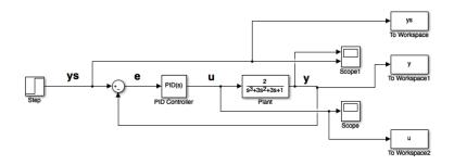
Figure 3.15: Block diagram of the previously mentioned example system in figure 3.4 implementing a proportional-integrative-derivative control. Being e the control error,  $y_s$  the target or expected value for the control variable, y the control variable and u the output of the controller.
