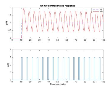
Figure 3.7: Response of the closed-loop system with an On-Off control. The transfer function of the process is  $G(s) = 2 \cdot (s+1)^{-3}$  with set-point of  $y_s = 1$ . Being y(t) the control variable and u(t) the output of the controller ( $u_{max} = 3$  and  $u_{min} = 0$ ).
