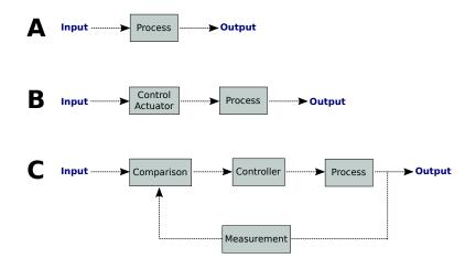
Figure 3.2: Block diagrams of the main types of control systems. A) System or process to be controlled, B) Open-loop control system (without feedback) and C) Closed-loop control system (with feedback).
