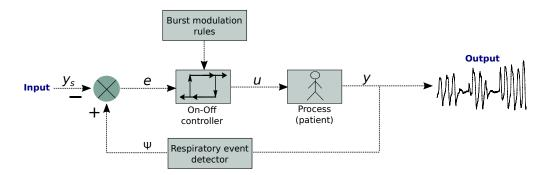
Figure 4.6: Block diagram of the PASITHEA system integrating an "on-off" controller, being,  $y_s$  the set-point or expected value, e the error, u the output of the controller, y the output of the system which, in this case is the patient, and its output the nasal pressure (NP) signal, and  $\Psi$  the output of the respiratory event detector.
