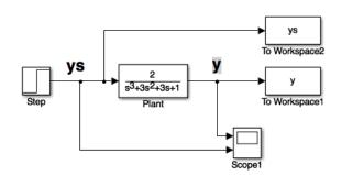
Figure 3.4: Open loop block diagram of the system to be controlled with a transfer function  $G(s) = 2 \cdot (s+1)^{-3}$ .
