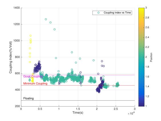
Figure 7.10: Example of mechanical coupling estimation for a complete night of recording. The black, red and violet lines represent the different coupling thresholds. Body positions are represented by a color-bar, 1) yellow = the head of the patient rests on top of the actuator, 2) green = neutral position where the actuator is on one side of the head without any other contact and 3) blue = the actuator is on the opposite side to the resting place of the head of the patient.
