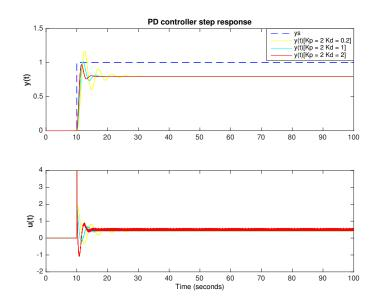
Figure 3.14: Response of the closed-loop system with proportional-derivative (PD) control. The transfer function of the process is  $G(s) = 2 \cdot (s+1)^{-3}$  with set-point of  $y_s = 1$ . Being y(t) the control variable and u(t) the output of the controller. Responses to fixed proportional gains  $(K_p)$  for different derivative coefficients  $(K_d)$  are shown.
