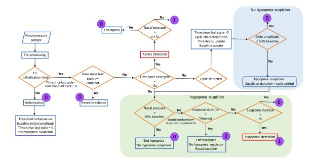
Figure 4.7: Block diagram of the functioning of the proposed real-time respiratory event detector. The input is the nasal pressure (NP) signal sampled at a frequency of 1/Ts (typically 8-200 Hz). The output is a signal  $\Psi$  with the same sample frequency with binary values between 0 and 1 (0 = no event detected and 1 = presence of a respiratory event). Adapted frigure from (FEUERSTEIN et al., 2015).
