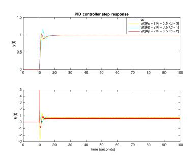
Figure 3.16: Response of the closed-loop system with proportional-integrative-derivative (PID) control. The transfer function of the process is  $G(s) = 2 \cdot (s+1)^{-3}$  with set-point of  $y_s = 1$ . Being y(t) the control variable and u(t) the output of the controller. Responses to fixed proportional gains  $(K_p)$  and integrative coefficients  $(K_i)$  for different derivative coefficients  $(K_d)$  are shown.
