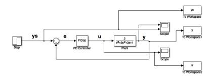
Figure 3.13: Block diagram of the previously mentioned example system in figure 3.4 implementing a proportional-derivative control. Being e the control error,  $y_s$  the target or expected value for the control variable, y the control variable and u the output of the controller.
