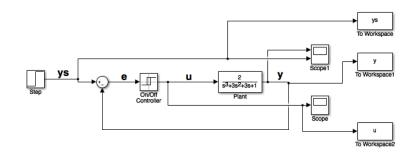
Figure 3.6: Block diagram of the previously mentioned example system in figure 3.4 implementing an on-off control. Being e the control error,  $y_s$  the target or expected value for the control variable, y the control variable and u the output of the controller.
