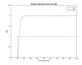
Figure 3.5: System response to the unit step in open loop, converging to a value of 2 in steady state.
