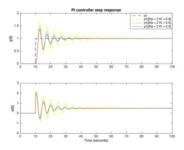
Figure 3.12: Response of the closed-loop system with proportional-integrative (PI) control. The transfer function of the process is  $G(s) = 2 \cdot (s+1)^{-3}$  with set-point of  $y_s = 1$ . Being y(t) the control variable and u(t) the output of the controller. Responses to fixed proportional gains  $(K_p)$  for different integral coefficients  $(K_i)$  are shown.
