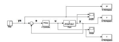
Figure 3.8: Block diagram of the previously mentioned example system in figure 3.4 implementing an on-off control. Being e the control error,  $y_s$  the target or expected value for the control variable, y the control variable and u the output of the controller.
