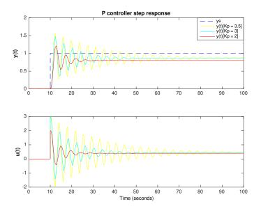
Figure 3.9: Response of the closed-loop system with proportional (P) control. The transfer function of the process is  $G(s) = 2 \cdot (s+1)^{-3}$  with set-point of  $y_s = 1$ . Being y(t) the control variable and u(t) the output of the controller. Responses to different proportional gains  $(K_p)$  are shown.
