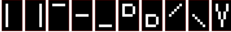
Figure 4.6: The 10 features that are used in Table 4.1. From the left to the right of the figure: left vertical bar, right vertical bar, top horizontal bar, middle horizontal bar, bottom horizontal bar, top belly, bottom belly, top diagonal bar, bottom diagonal bar, double diagonal bar.
