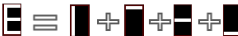
Figure 4.5: The letter E can be built by super-imposing four different strokes, three horizontal bars (top, middle, and bottom) and one vertical bar (left).
