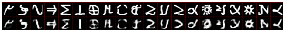
Figure 10.5: Inputs and reconstructions of samples from the HWRT dataset (Thoma, 2015) obtained using a denoising autoencoder trained on MNIST. Input images are in the first row. The corresponding reconstructed images are in the second row.
