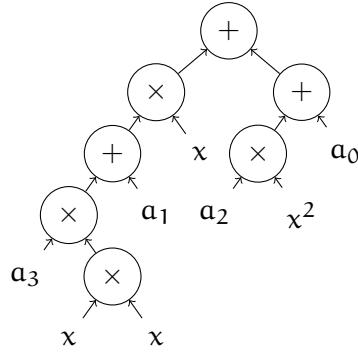
Figure 3.2 – Second-order Horner’s scheme for a degree-3 polynomial.
