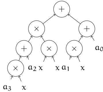
Figure 3.3 – Estrin’s scheme for a degree-3 polynomial.
