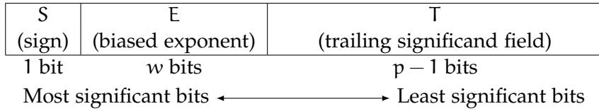
Figure 1.1 – IEEE 754 Binary Interchange Floating-Point Format.
