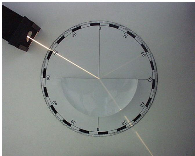
Figure 1 – Refraction of light at the interface between air and PMMA. Credit: Zátónyi Sándor, <https://commons.wikimedia.org/wiki/File:Fénytörés.jpg>, CC-BY-SA 3.0.
