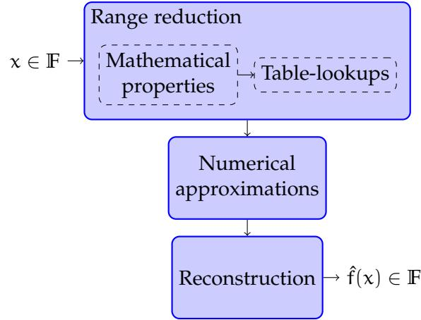
Figure 1.3 – Overview of a typical evaluation scheme for an elementary function  $x \mapsto f(x)$ . Note that it results in  $\hat{f}(x)$ , and not in  $f(x)$ , as it is an approximation in finite-precision arithmetic.
