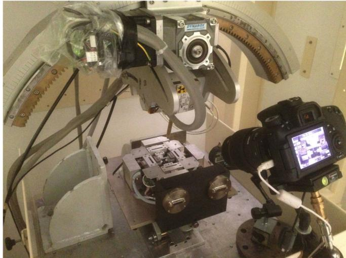
FIGURE 2.6 – *In-situ* tensile test enabling for XRD stress analyses
