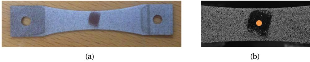
FIGURE 2.9 – Coupon for *in-situ* tests. (a) Dog-bone geometry (ligament width : 6 mm, thickness : 0.5 mm, radius of the hour-glass shape : 65 mm). (b) Speckle pattern used for DIC procedures with an unpainted area to allow for XRD measurements. The area probed by the X-ray beam is depicted in orange.
