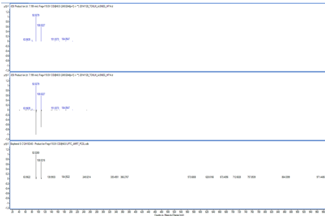
Figure S5. Comparison of fragmentation spectrum of suspect compounds present in F1, F2 with analytical standard (Bisphenol S)
