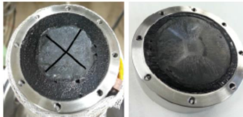
Figure 1. YBCO (left) and GdBCO (right) bulk superconductor samples. The growth sector boundaries (GSBs) are shown in each sample.
