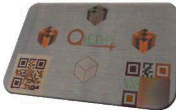
Figure 2.7: Marking “Qiova” and two-dimensional codes consisting of controlled nanostructures by femtosecond laser pulses on stainless steel [Qio16]
