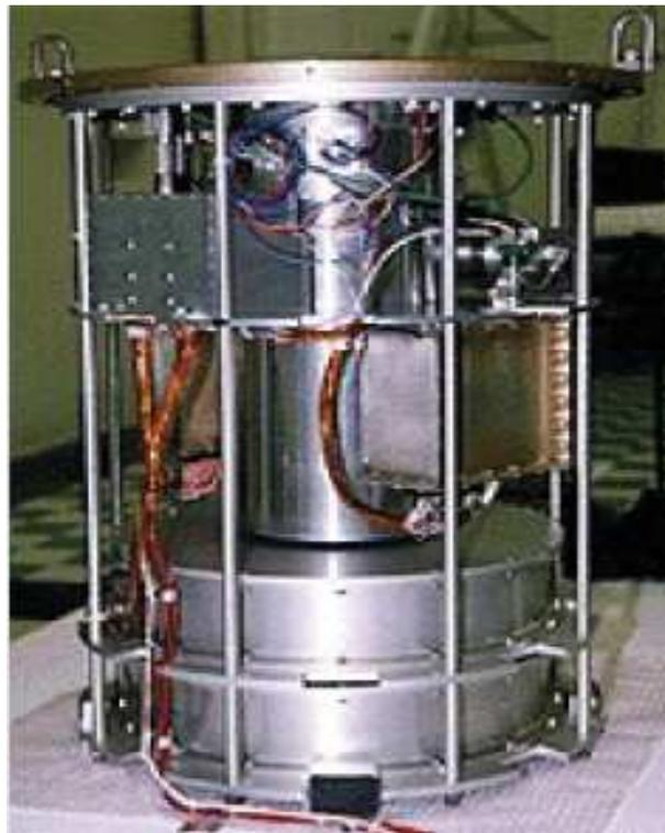
Figure 1.34: Space ThermoAcoustic Refrigerator [Star Penn State, 1992].
