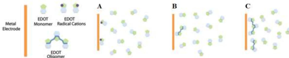
**Figure 2.** Electrical polymerization process. (a) The metal electrode oxidizes the EDOT monomers creating radical cations. (b) These radical cations combine, creating dimers, trimers, and higher oligomers. (c) As the molecular weight of the polymer chains increase they become insoluble, precipitating onto the metal electrode surface. Adapted with permission.<sup>[8]</sup> Copyright 2016, the Royal Society of Chemistry.
