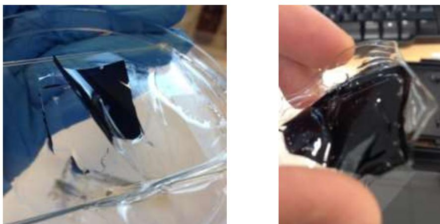
**Figure A.2.** Macroscopic images of big area patterned PEDOT:PSS film demolded from a PDMS mold using PVA layer.
