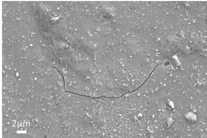
Figure 116 - Barrel surface of Virgo™38 after SSRT interrupted at 0.2% proof stress test at a strain rate of  $10^{-7}s^{-1}$  and under cathodic charging at -1200mV/SCE in a solution containing 30g/L NaCl + 0.4g/L sodium acetate at pH=1.5 (adjusted with HCl) purged with CO<sub>2</sub> with controlling the pH drift showing several secondary cracks
