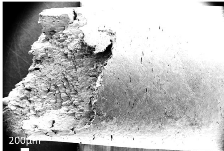
Figure 109 - Barrel surface of Virgo™38 after SSRT test at a strain rate of  $10^{-6} s^{-1}$  and under cathodic charging at  $-1200mV/SCE$  in a solution containing 30g/L NaCl + 0.4g/L sodium acetate at  $pH=1.5$  (adjusted with HCl) purged with  $CO_2$  showing several secondary cracks
