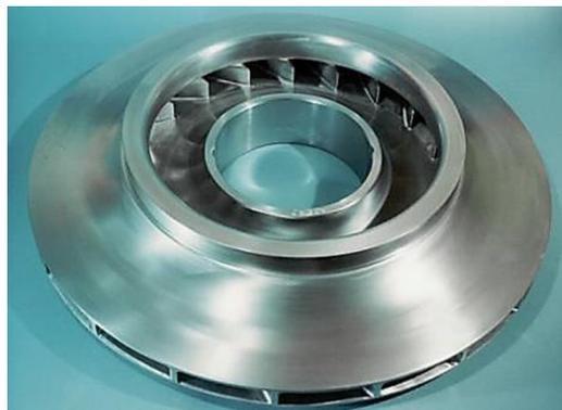
Figure 2 - Centrifugal compressor impeller
