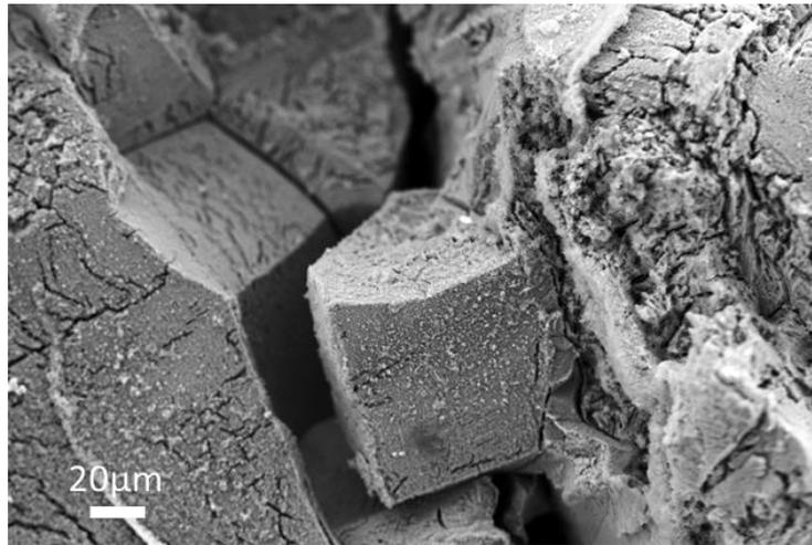
Figure 209 - Fracture surface obtained after SSRT test on the Cover sample tested under 1 bar of H<sub>2</sub>S, in presence of 600ppm of chlorides at pH=3.5 and at a strain rate of 10<sup>-7</sup>s<sup>-1</sup> showing a fully intergranular fracture
