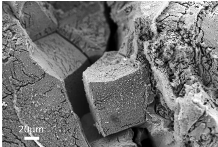
Figure 209 - Fracture surface obtained after SSRT test on the Cover sample tested under 1 bar of H 2 S, in presence of 600ppm of chlorides at pH=3.5 and at a strain rate of 10 -7 s -1 showing a fully intergranular fracture
