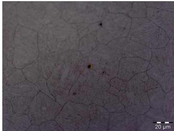
Figure 191 - Optical micrograph of a sample mirror polished after 30min immersion at the Open Circuit Potential in a solution containing 30g/L NaCl + 0.4g/L sodium acetate at pH=1.5 showing pitting corrosion of TiC
