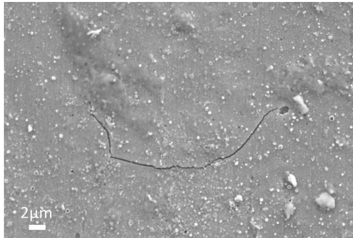
Figure 116 - Barrel surface of Virgo™38 after SSRT interrupted at 0.2% proof stress test at a strain rate of 10^{-7}s^{-1} and under cathodic charging at -1200mV/SCE in a solution containing 30g/L NaCl + 0.4g/L sodium acetate at pH=1.5 (adjusted with HCl) purged with CO 2 with controlling the pH drift showing several secondary cracks
