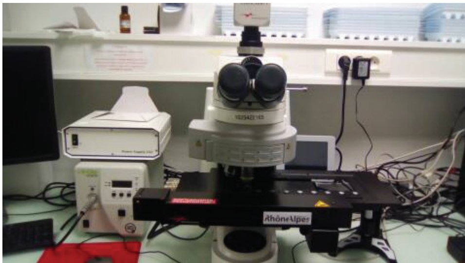
Figure 57: The Metafer platform used for \gamma H2AX analysis along with the microscope (Lyon-Sud Medical School).
