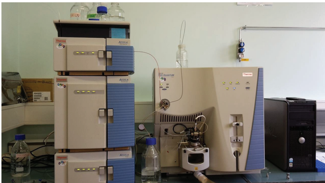
Figure 58: Photograph of the HPLC coupled to a MS/MS for detection of 8-oxo-guanine (INAC/SyMMES/CIBEST, CEA-Grenoble, Grenoble, France).
