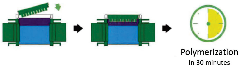
Figure 55: Schematic representation of the three different steps for the preparation of the gel for Western-Blot.
