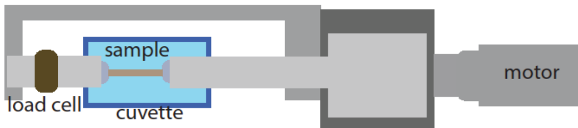
Fig 3.2.5: In the tensile stage the sample is fixed in between two clamps and fully immersed in solution. Setup's main components are: a load cell (in brown) to control and measure axial tensile forces, and a linear motor (on the right part of a strain) to control and measure the strain.
